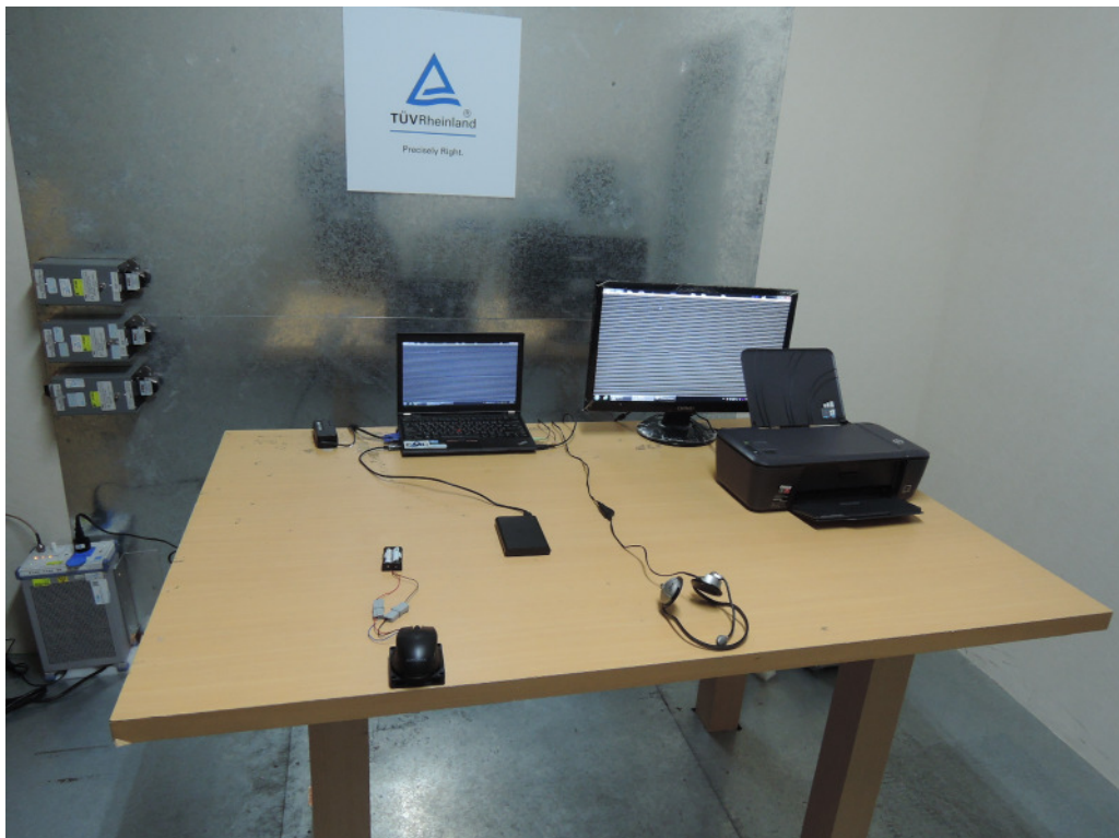
Photograph 5: Set-up for for Mains Conducted testing Front
