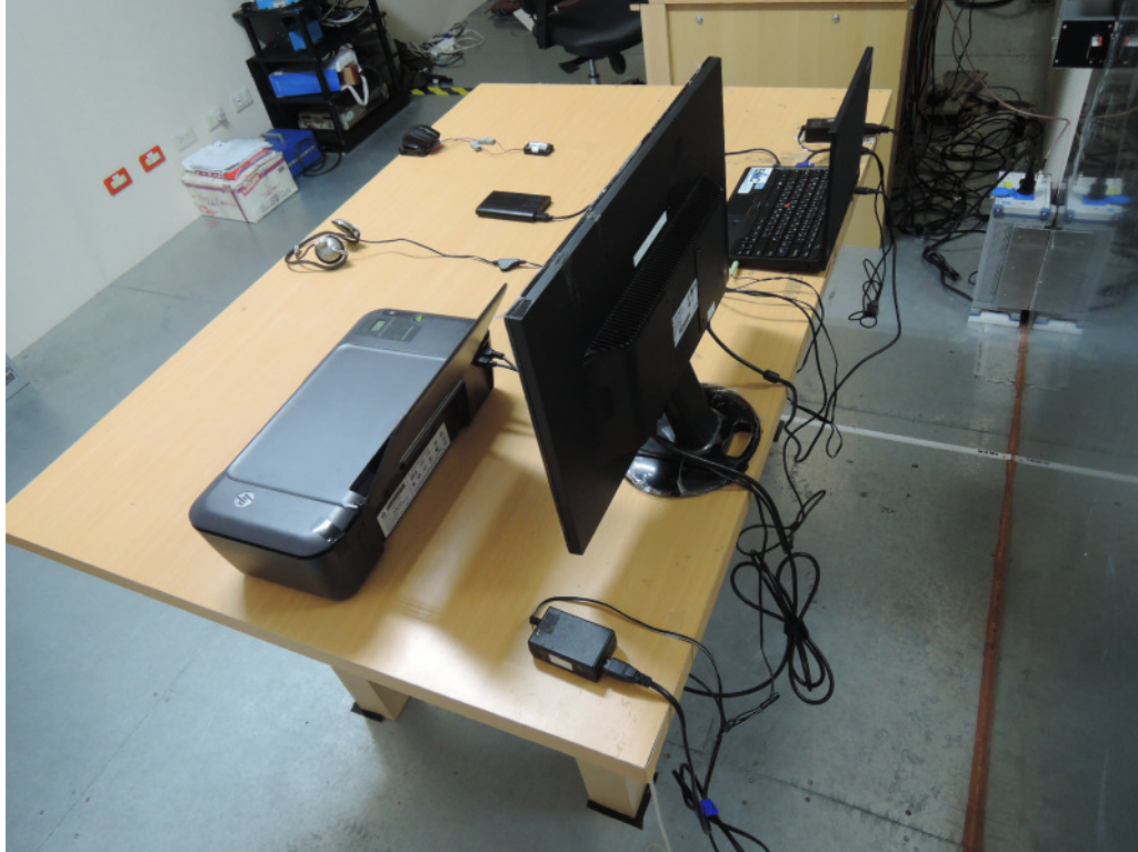
Photograph 4: Set-up for for Mains Conducted testing Back
