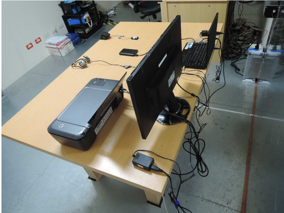
Photograph 4: Set-up for for Mains Conducted testing Back
