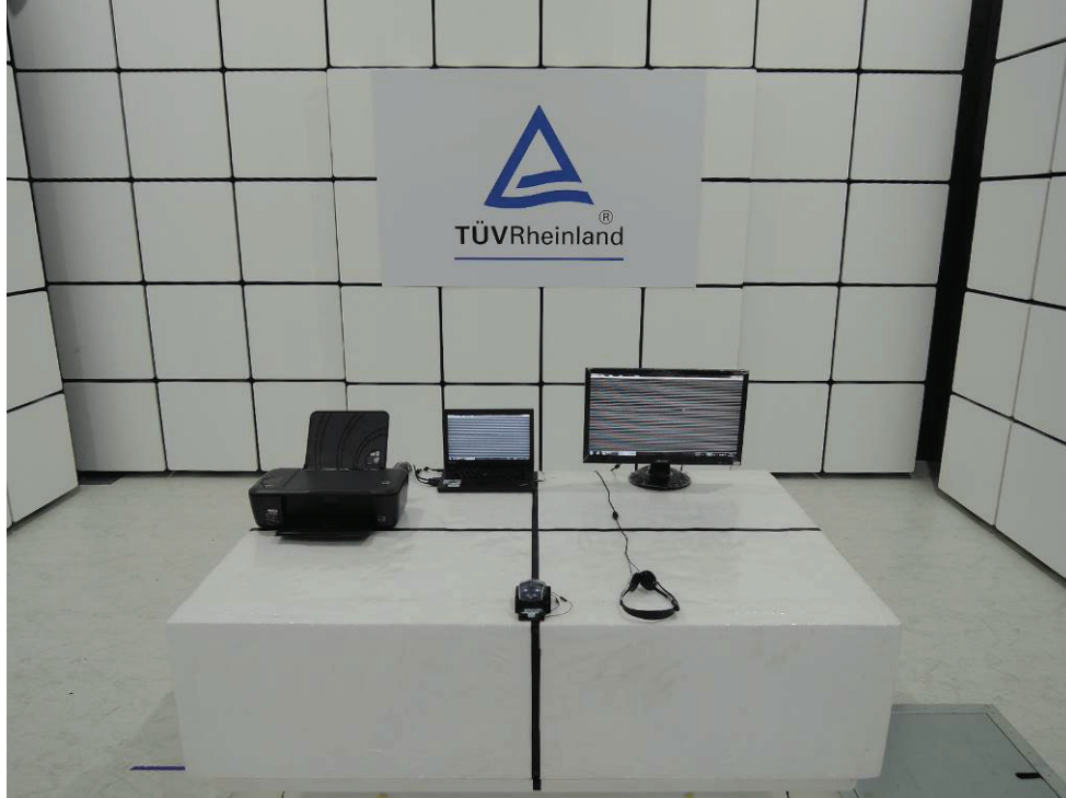
Picture 3: Radiated Emission, Above 1 GHz
