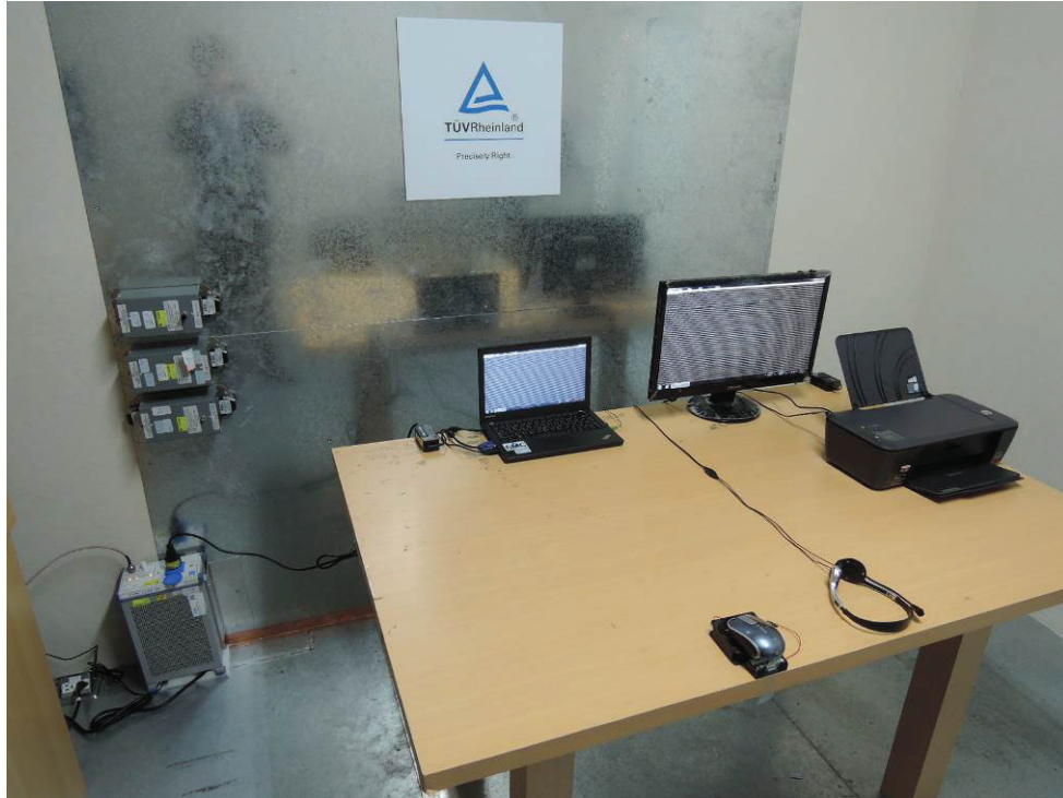
Picture 1: Conducted Emission, AC Mains; 0.15 – 30 MHz
