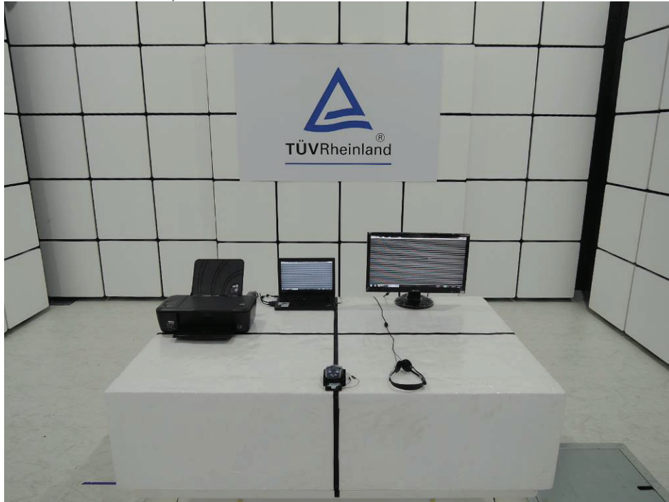
Picture 2: Radiated Emission, 30 - 1000 MHz
