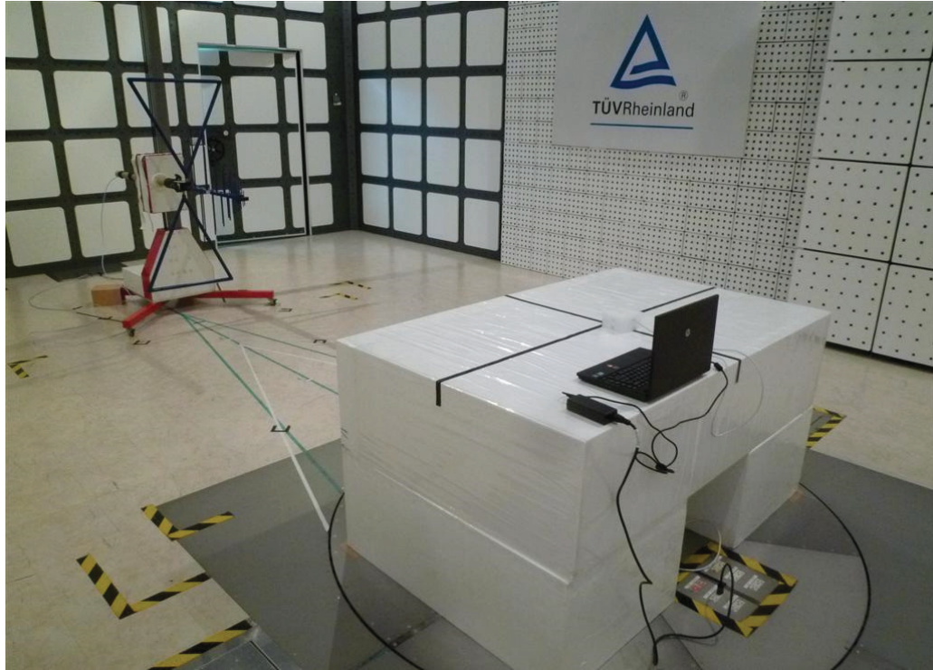
Photograph 3: Set-up for Spurious Emissions (Back View 2 TX)
