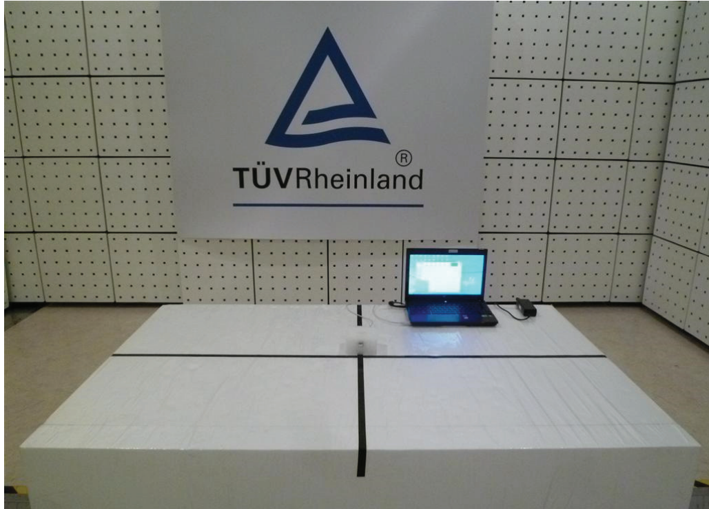
Photograph 1: Set-up for Spurious Emissions (Front View)
