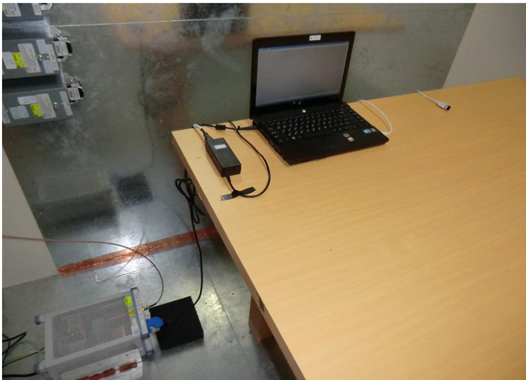
Photograph 5: Set-up for for Mains Conducted testing Front
