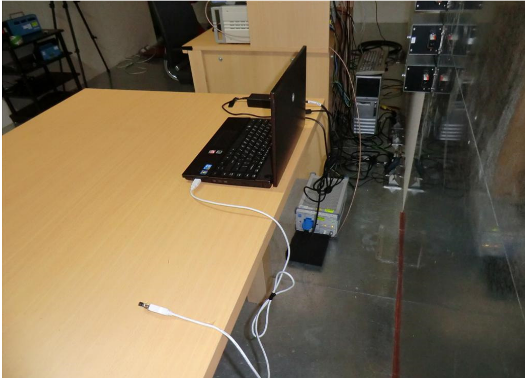
Photograph 4: Set-up for for Mains Conducted testing Back
