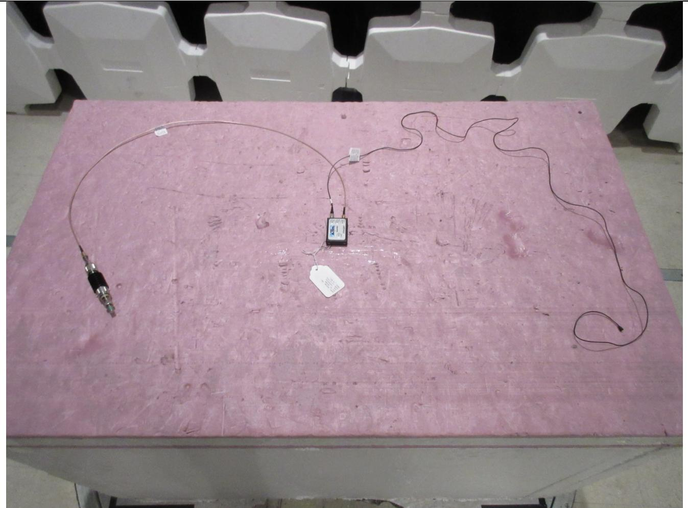
FIELD STRENGTH OF SPURIOUS EMISSIONS BELOW 30 MHz
