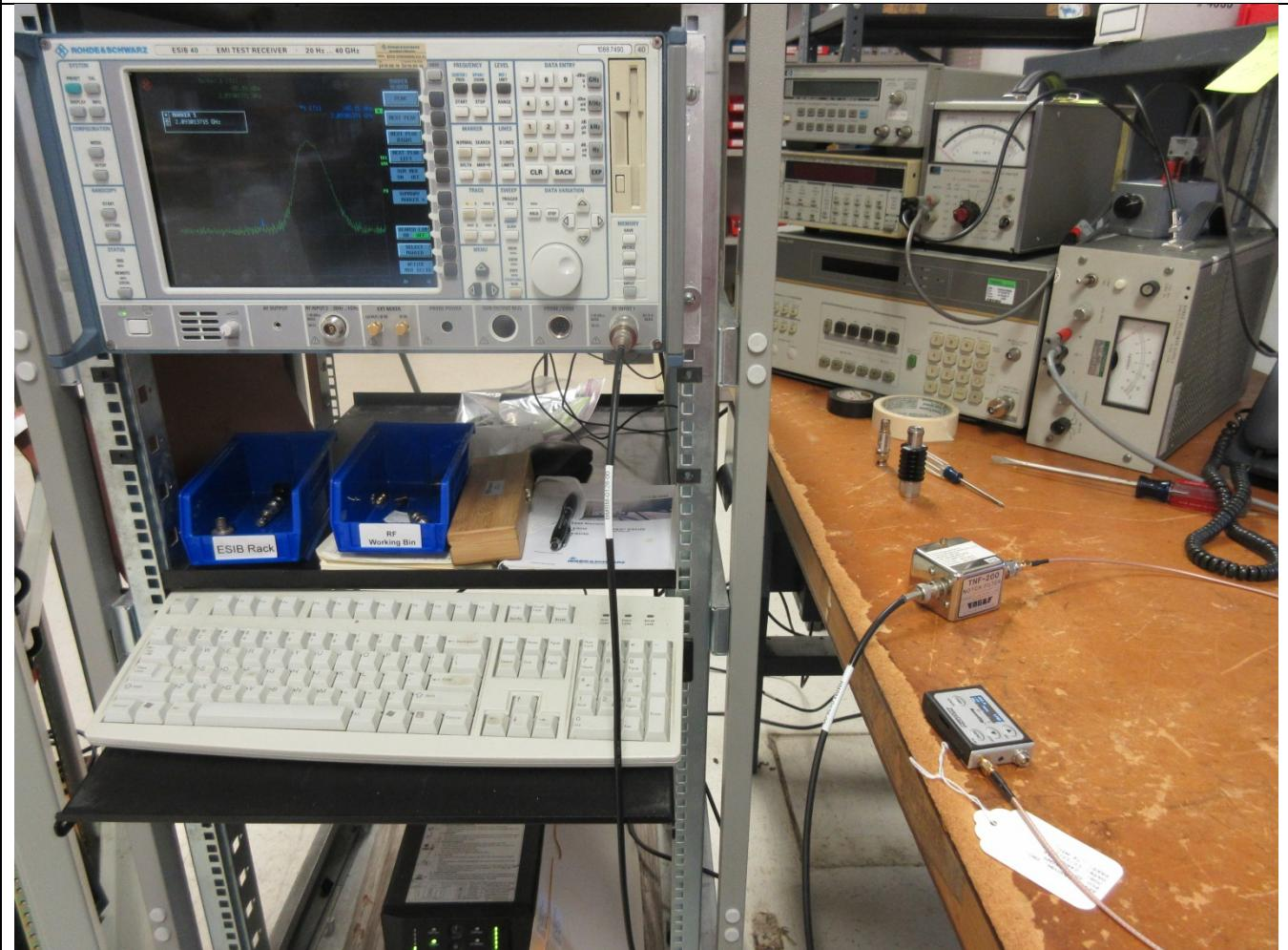
FIELD STRENGTH OF SPURIOUS EMISSIONS FINAL SETUP
