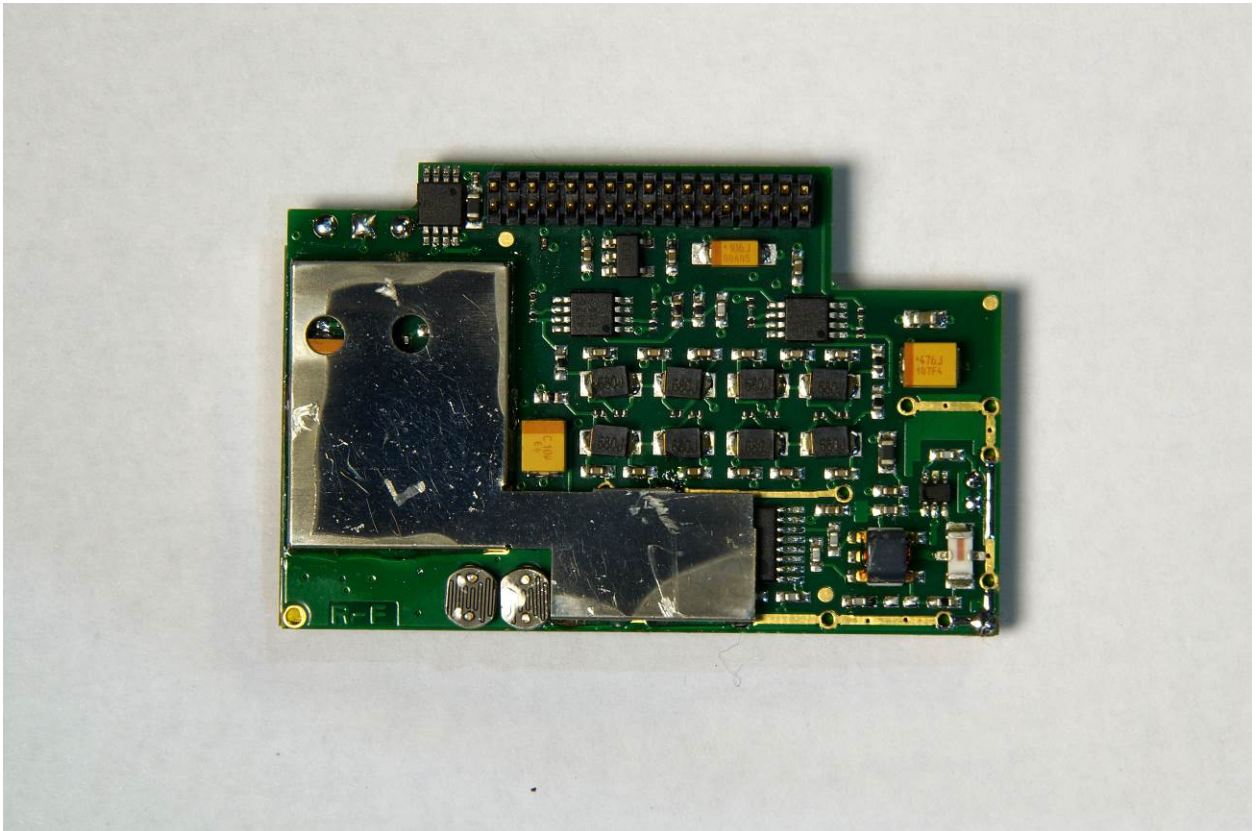
Figure 10: RF Board – Top View With Shielding
