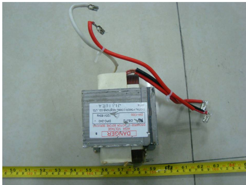
EUT - Transformer View
