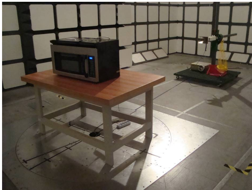
Radiated Emissions - Rear View (Above 1 GHz)
