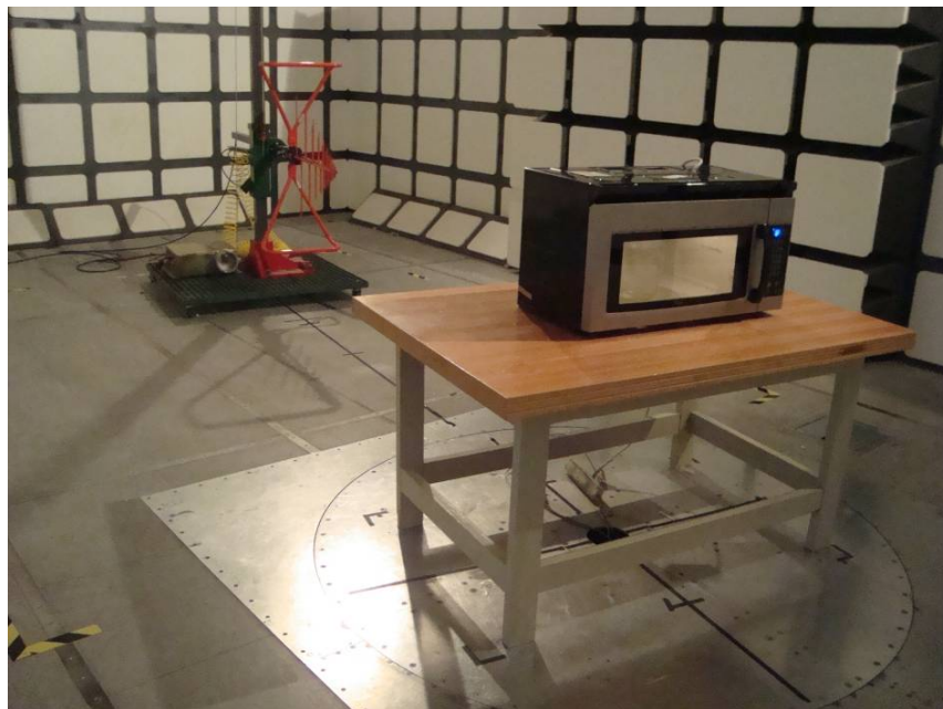
Radiated Emissions - Rear View (Below 1 GHz)
