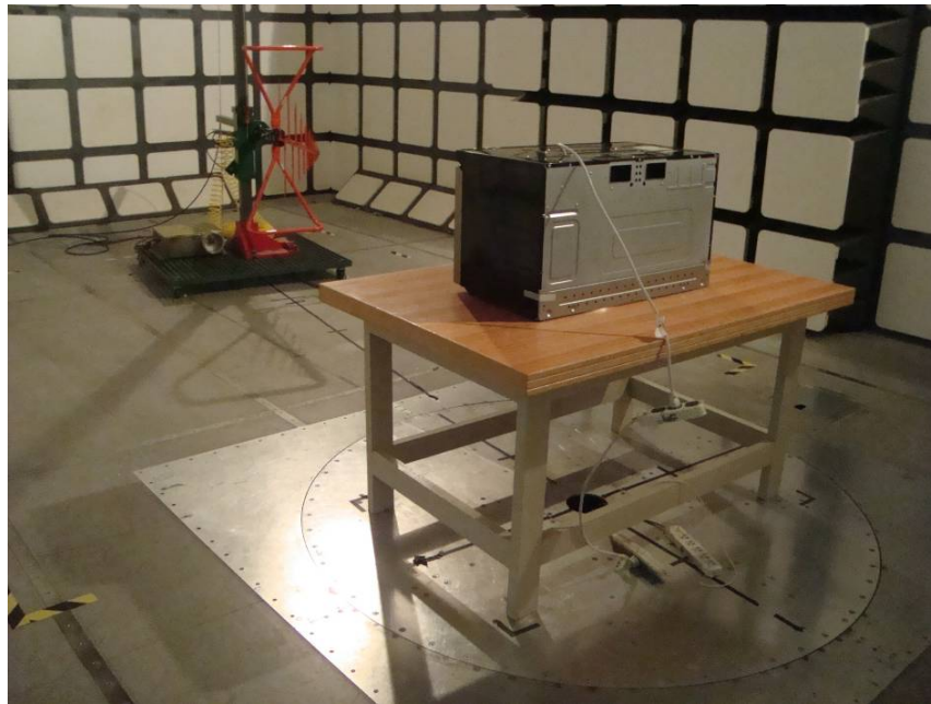
Radiated Emissions - Front View (Below 1 GHz)
