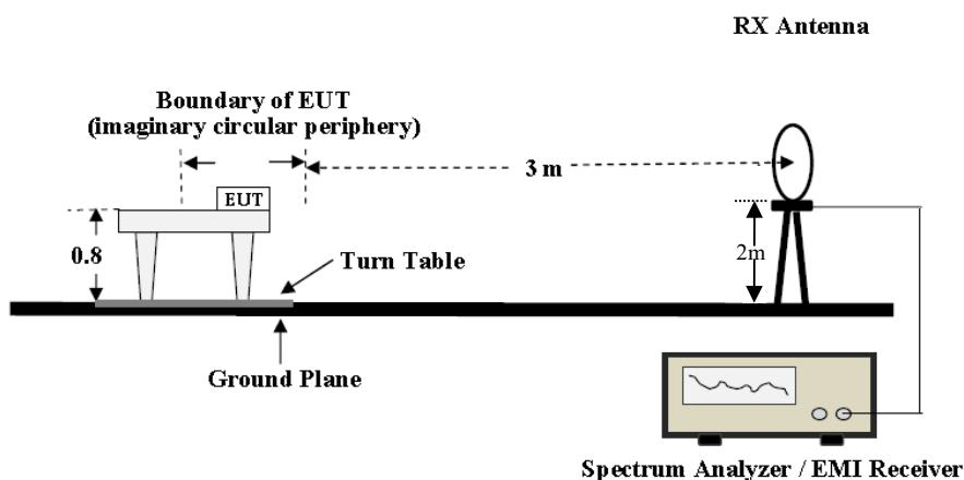
The radiated emission tests were performed in the 3 meters chamber test site, using the setup accordance with the FCC OST MP-5(1986). The related limit was specified in Part 18.305.
