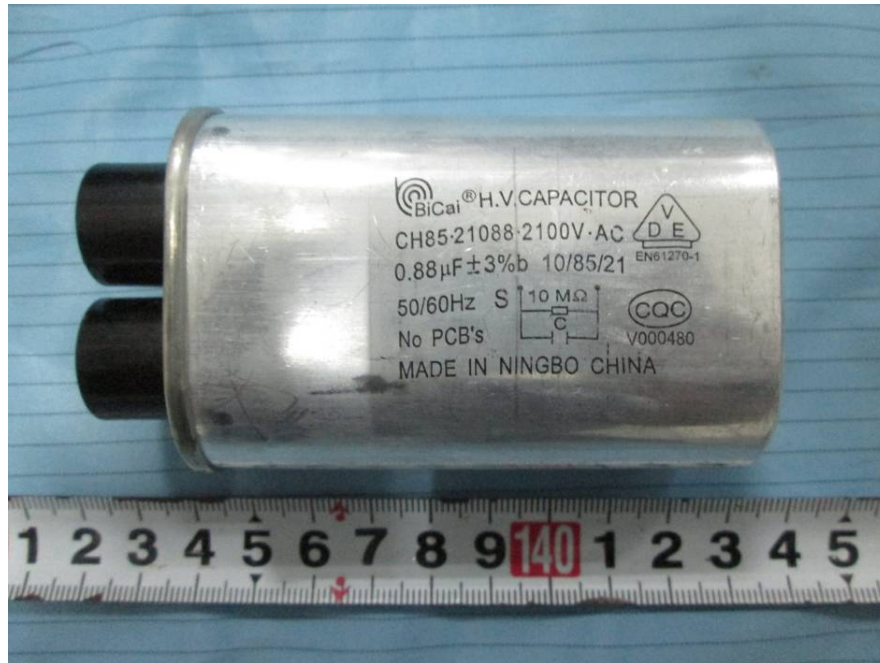
EUT – H.V. Capacitor View
