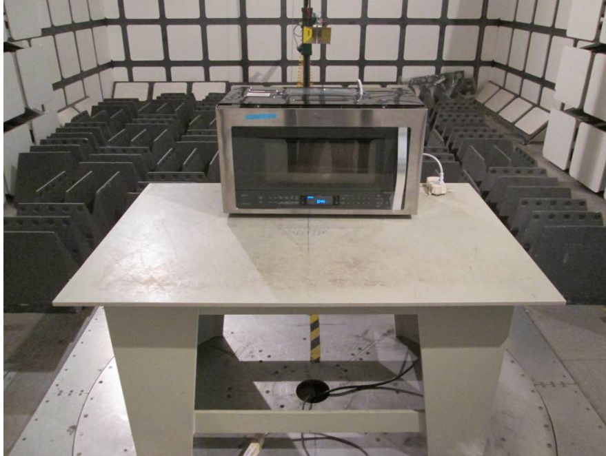
Radiated Emissions - Front View (Above 1 GHz)
