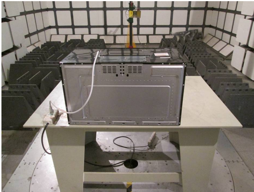
Radiated Emissions - Rear View (Above 1 GHz)
