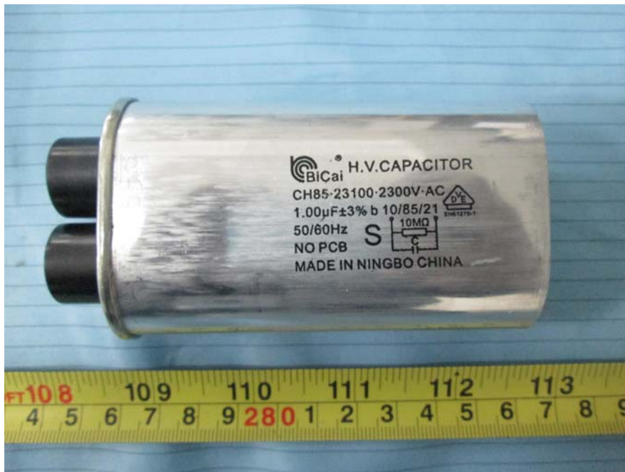
EUT – H.V. Capacitor View
