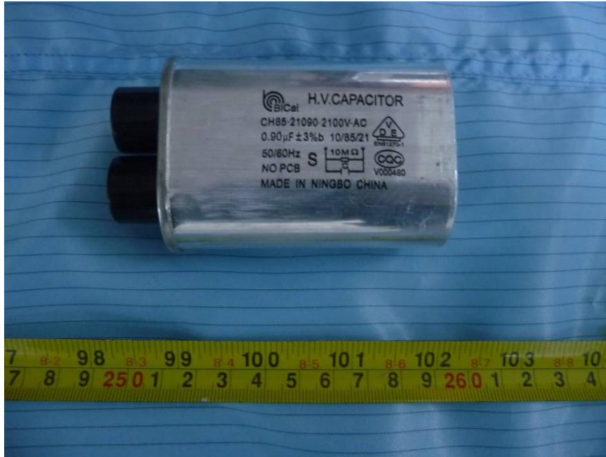
EUT – H.V. Capacitor View
