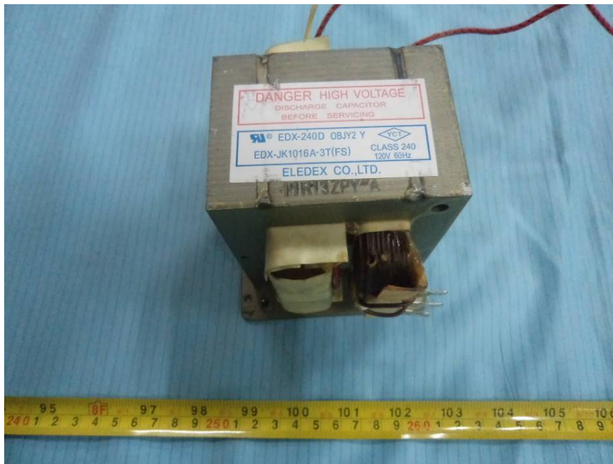
EUT – Power Transformer View
