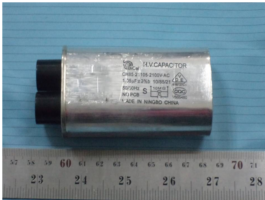
EUT – H.V. Capacitor View
