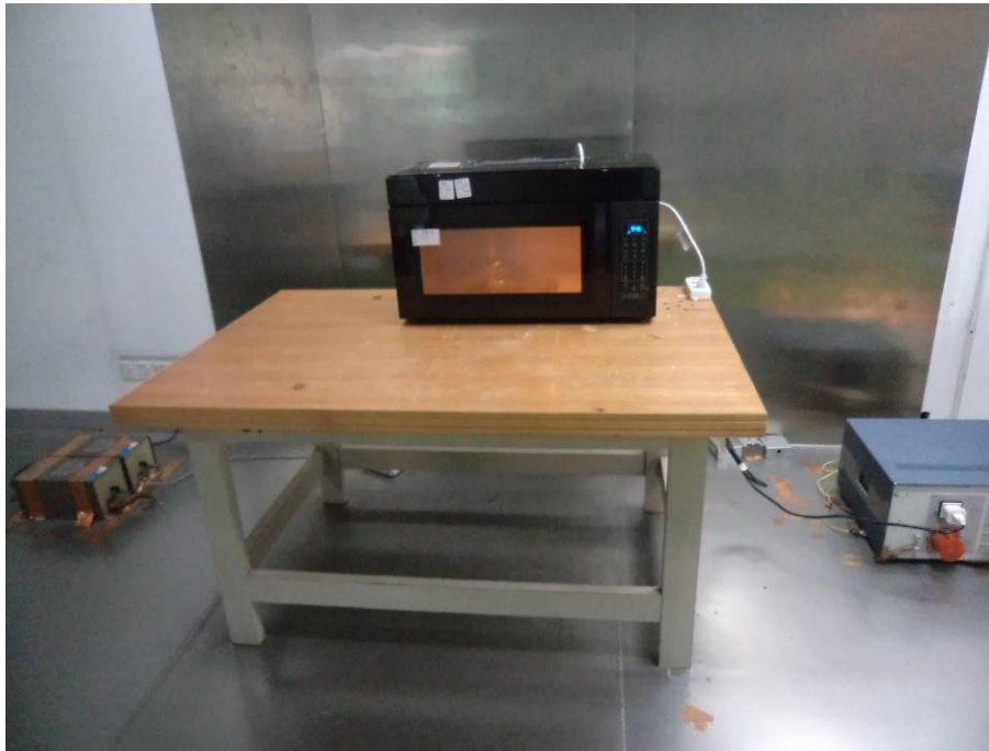
Conduction Emissions - Front View
