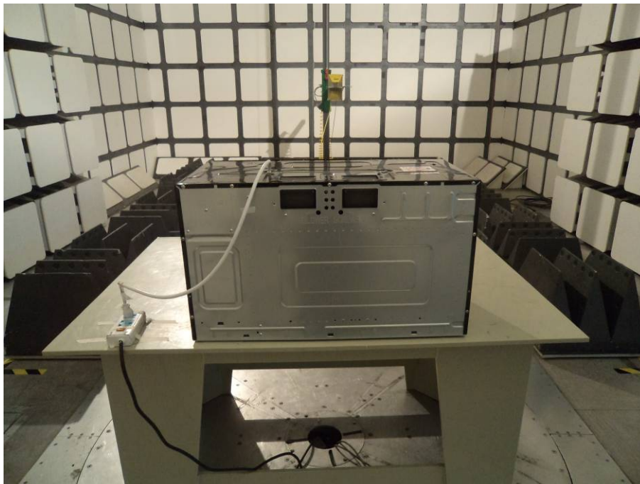
Radiated Emissions - Rear View (Above 1 GHz)
