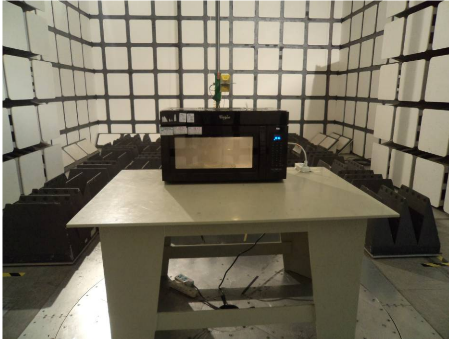
Radiated Emissions - Front View (Above 1 GHz)
