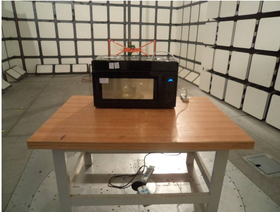
Radiated Emissions - Front View (Below 1 GHz)
