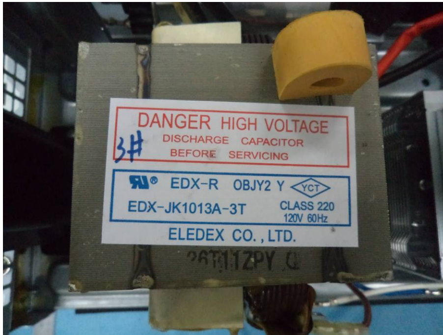
EUT – Transformer View
