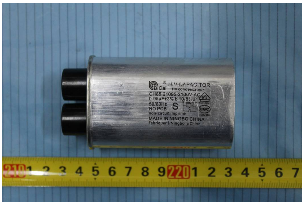
EUT –High Voltage Capacitor View
