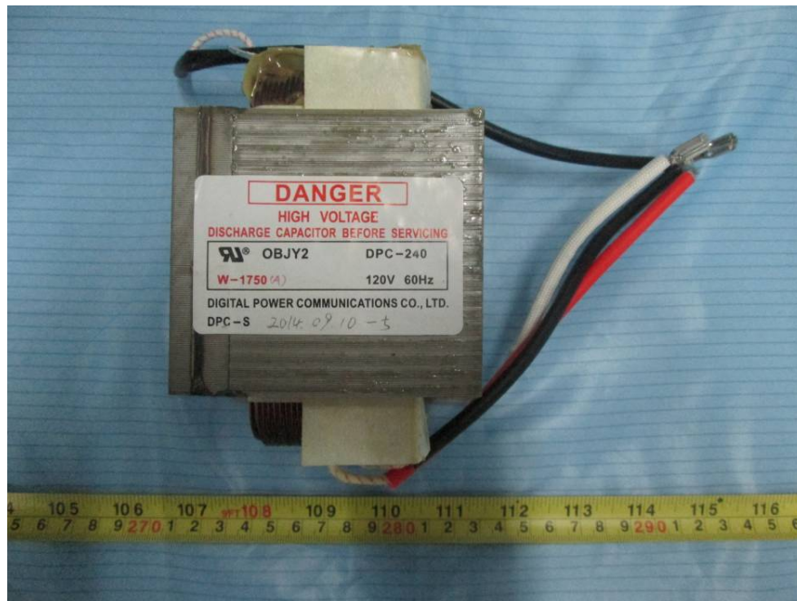
EUT – Power Transformer View
