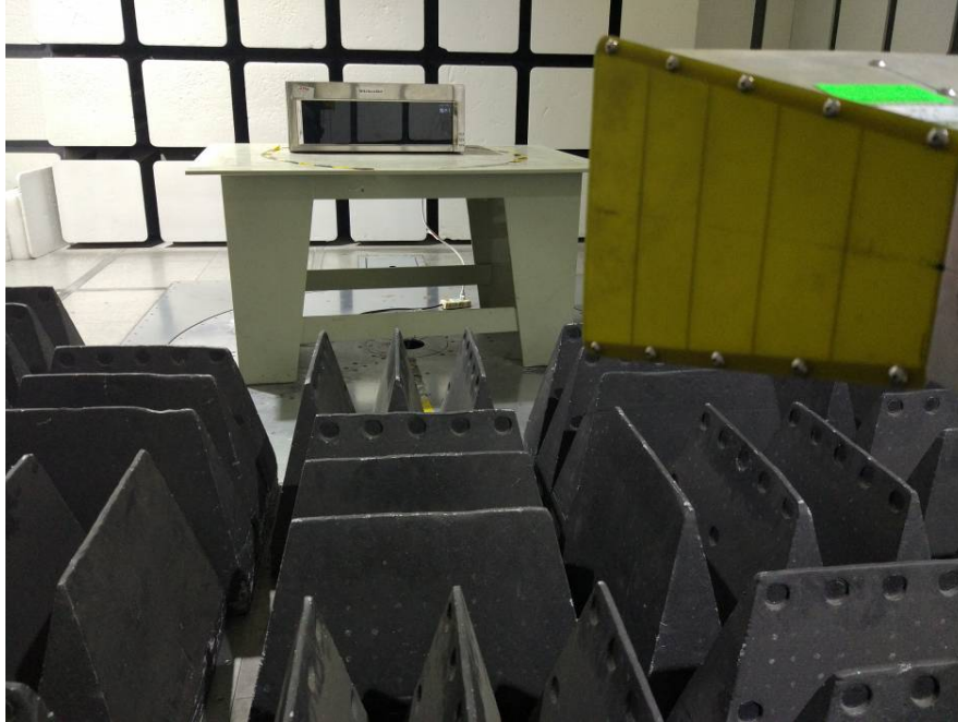
Radiated Emissions - Front View (Above 1 GHz)
