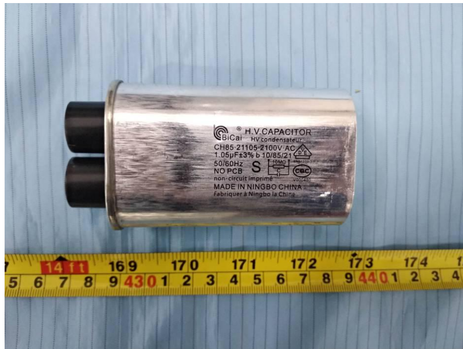
EUT – H.V. Capacitor Front View
