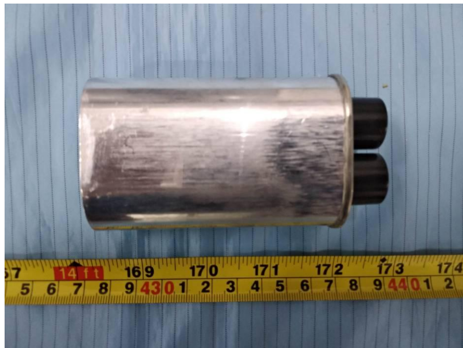
EUT – H.V. Capacitor Rear View
