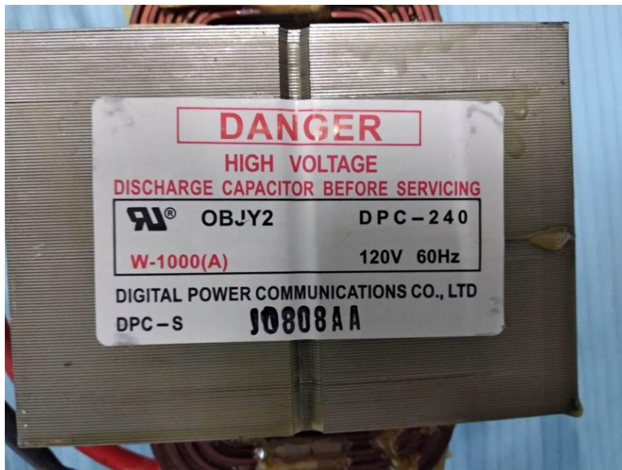
EUT – Transformer Label View
