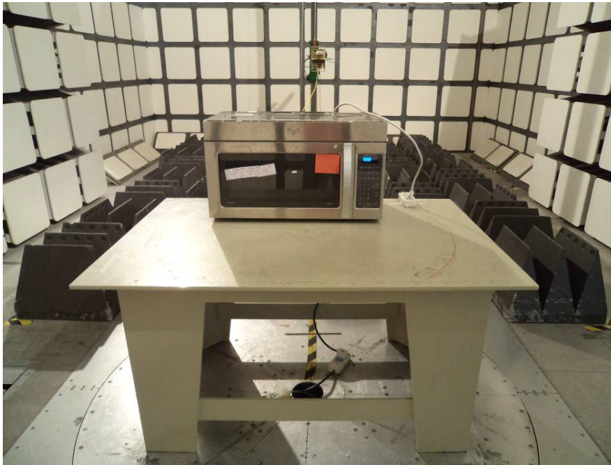
Radiated Emissions - Front View (Above 1 GHz)
