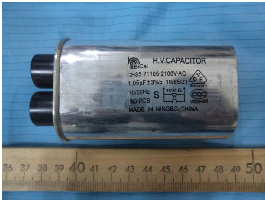
EUT – H.V. Capacitor View
