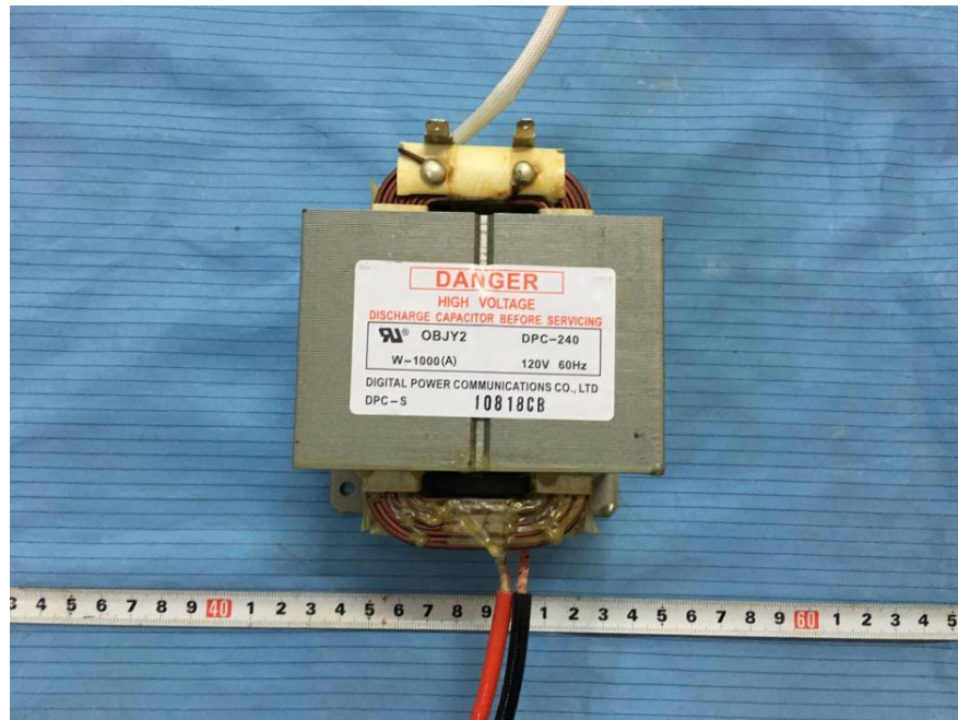
EUT – Transformer View
