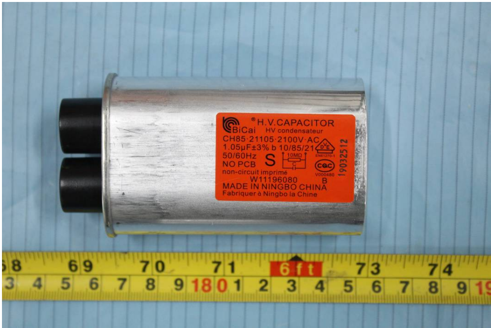
EUT –High Voltage Capacitor View
