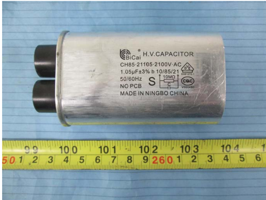
EUT – H.V. CAPACITOR View
