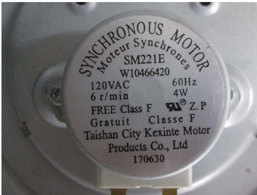
EUT – SYNCHRONOUS Motor View
