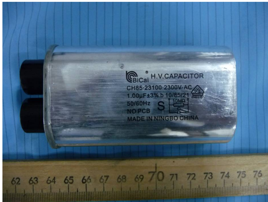
EUT – H.V. Capacitor View
