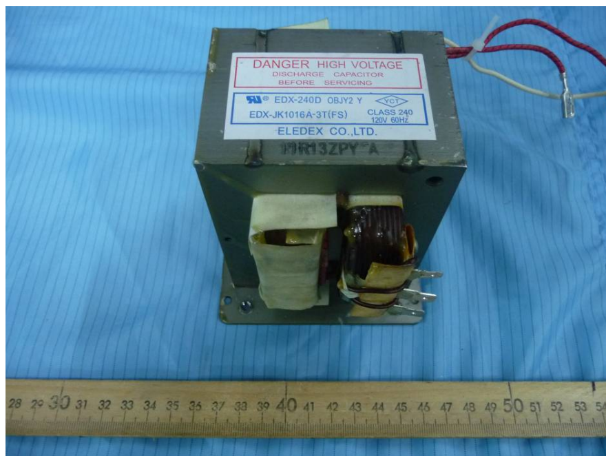
EUT – Power Transformer View
