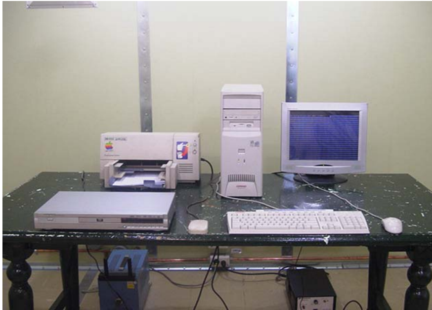
Photograph 2 : Setup for Conducted Emissions
