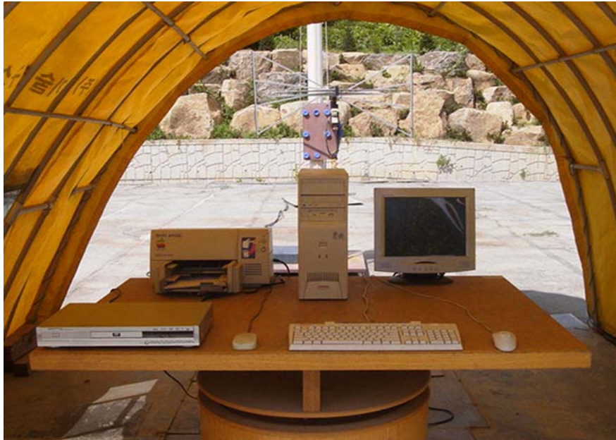
Photograph 1 : Setup for radiated Emissions
