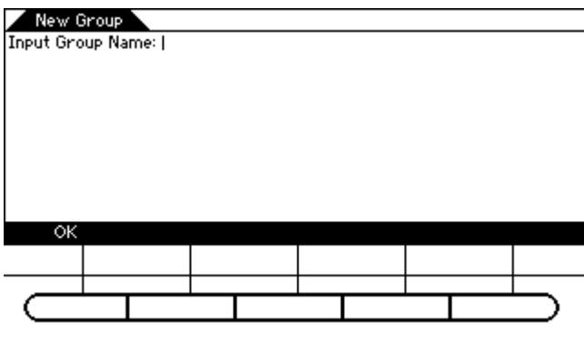
Press the **NAVIGATION** key indicating **NEW**, you can create an individual address and add it into the group address after you have saved it.
