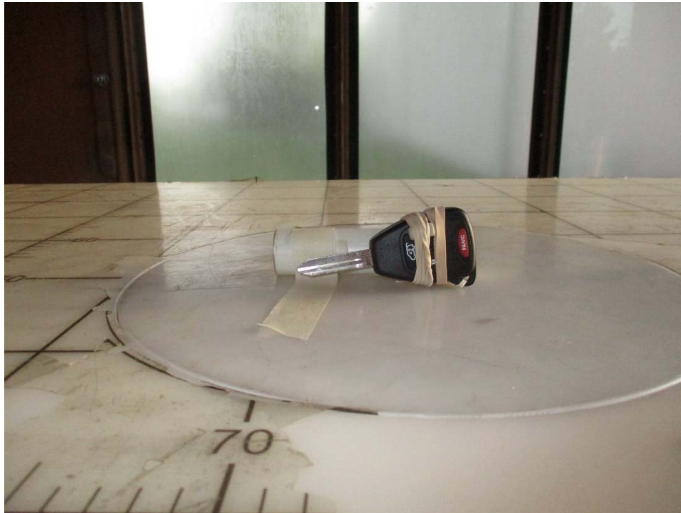
Test Setup, Y Axis, Below 1 GHz
