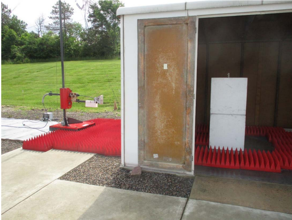
Horizontal Antenna Polarization, Above 1 GHz
