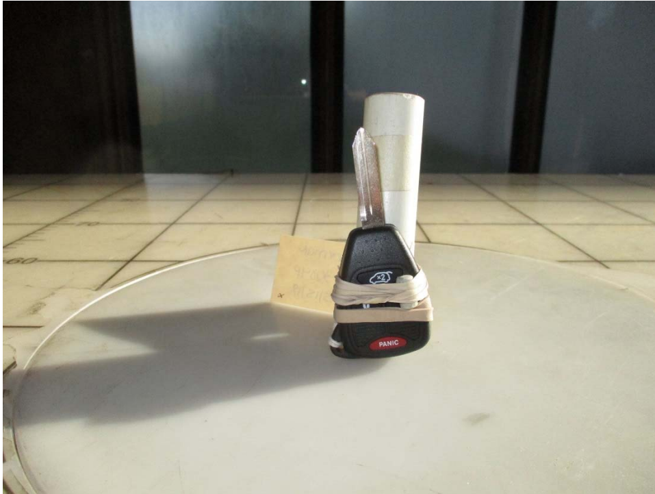
Test Setup, X Axis, Below 1 GHz
