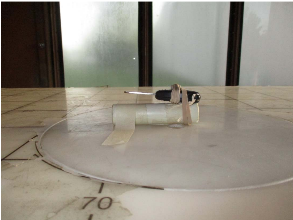
Test Setup, Z Axis, Above 1 GHz
