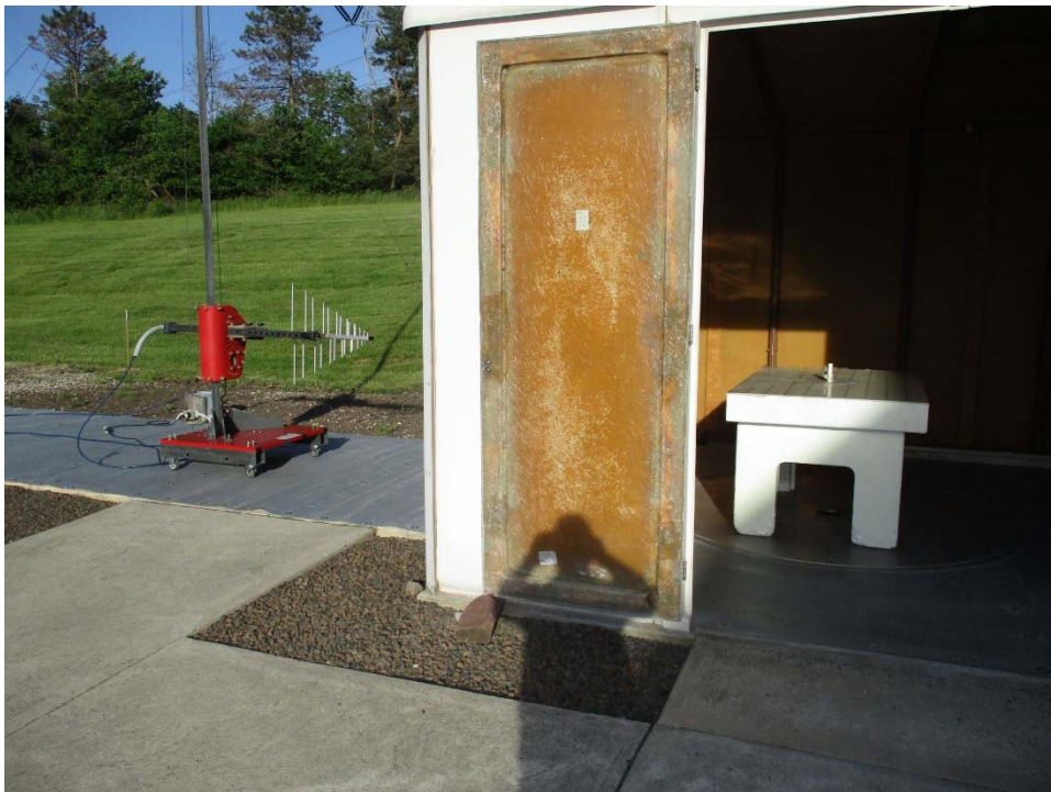
Vertical Antenna Polarization, Below 1 GHz
