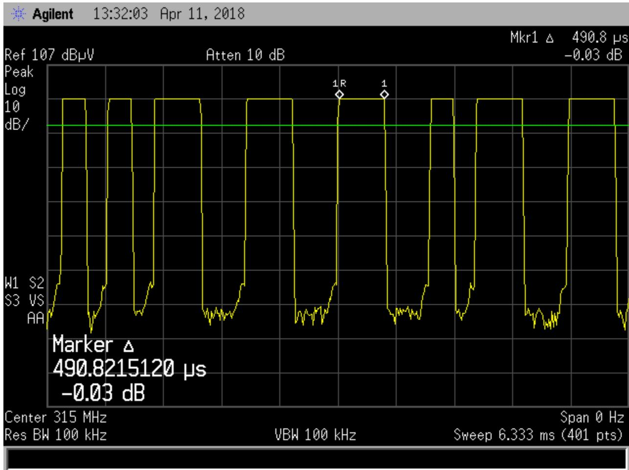
**Test Method: FCC Part 15.231(b), Duty Cycle Determination**
