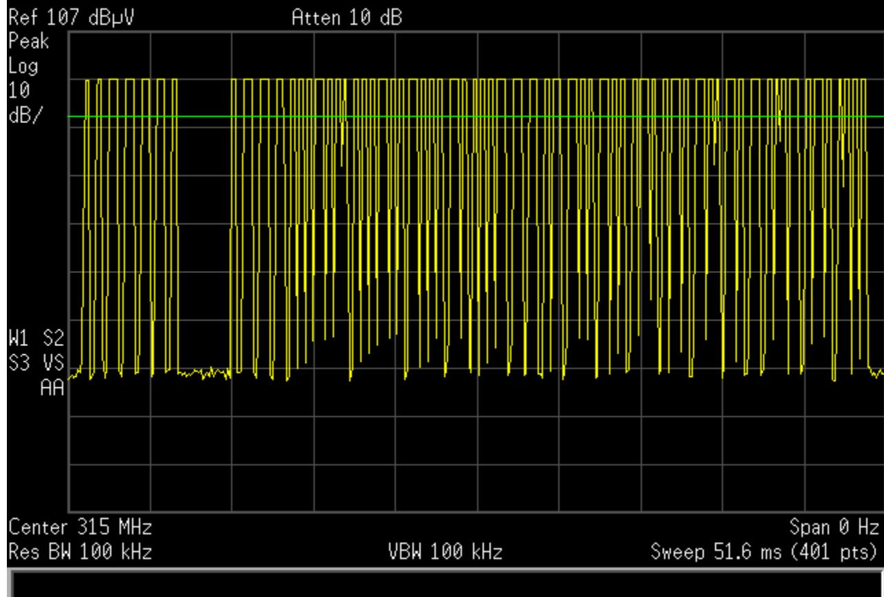
**Test Method: FCC Part 15.231(b), Duty Cycle Determination**
