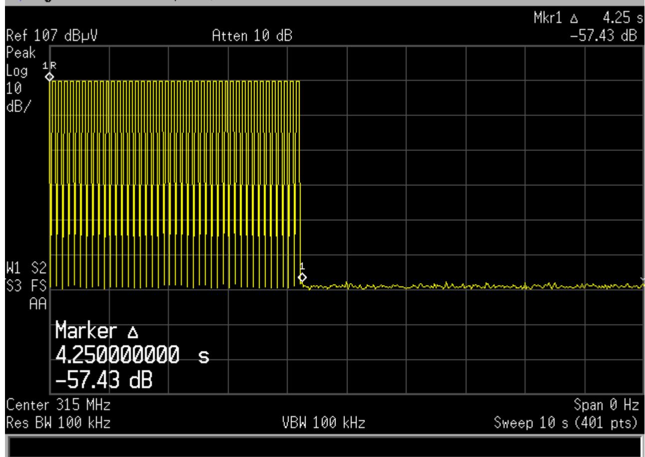
**Test Method: FCC Part 15.231(a)(1), Transmitter Deactivation Time**
