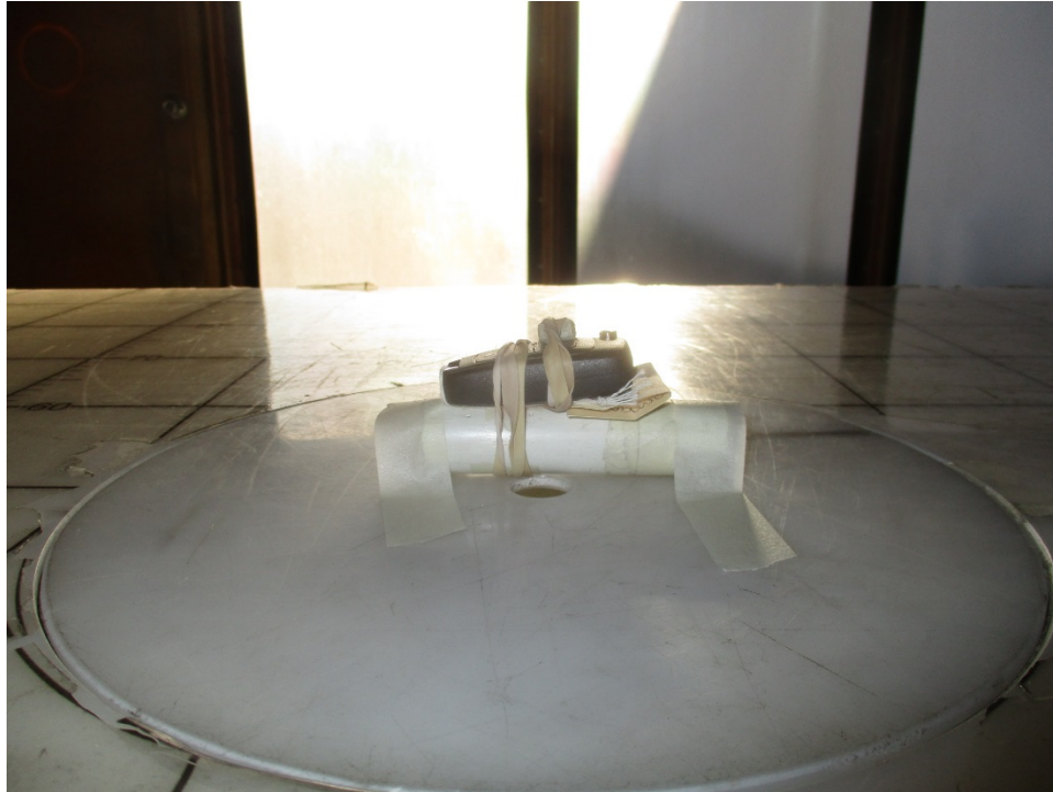
Test Setup, Z Axis, Below 1 GHz
