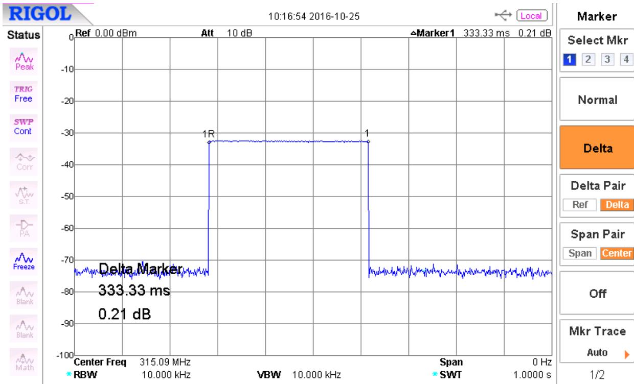
**Test Method: FCC Part 15.231(b), Duty Cycle Determination**
