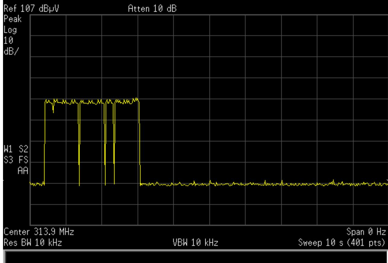
**Test Method: FCC Part 15.231(a)(1), Transmitter Deactivation Time**
