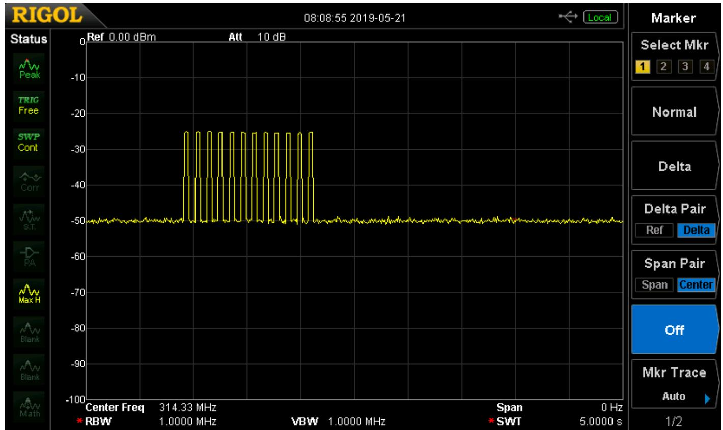
**Test Method: FCC Part 15.231(a)(1), Transmitter Deactivation Time**
