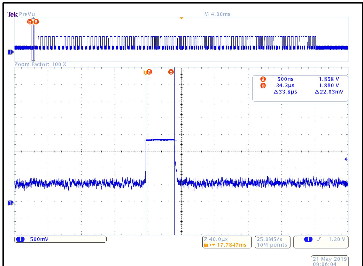
**Test Method: FCC Part 15.231(b)(2), Duty Cycle Determination IC RSS-210 A1.1.2(2) Pulsed Operation**
