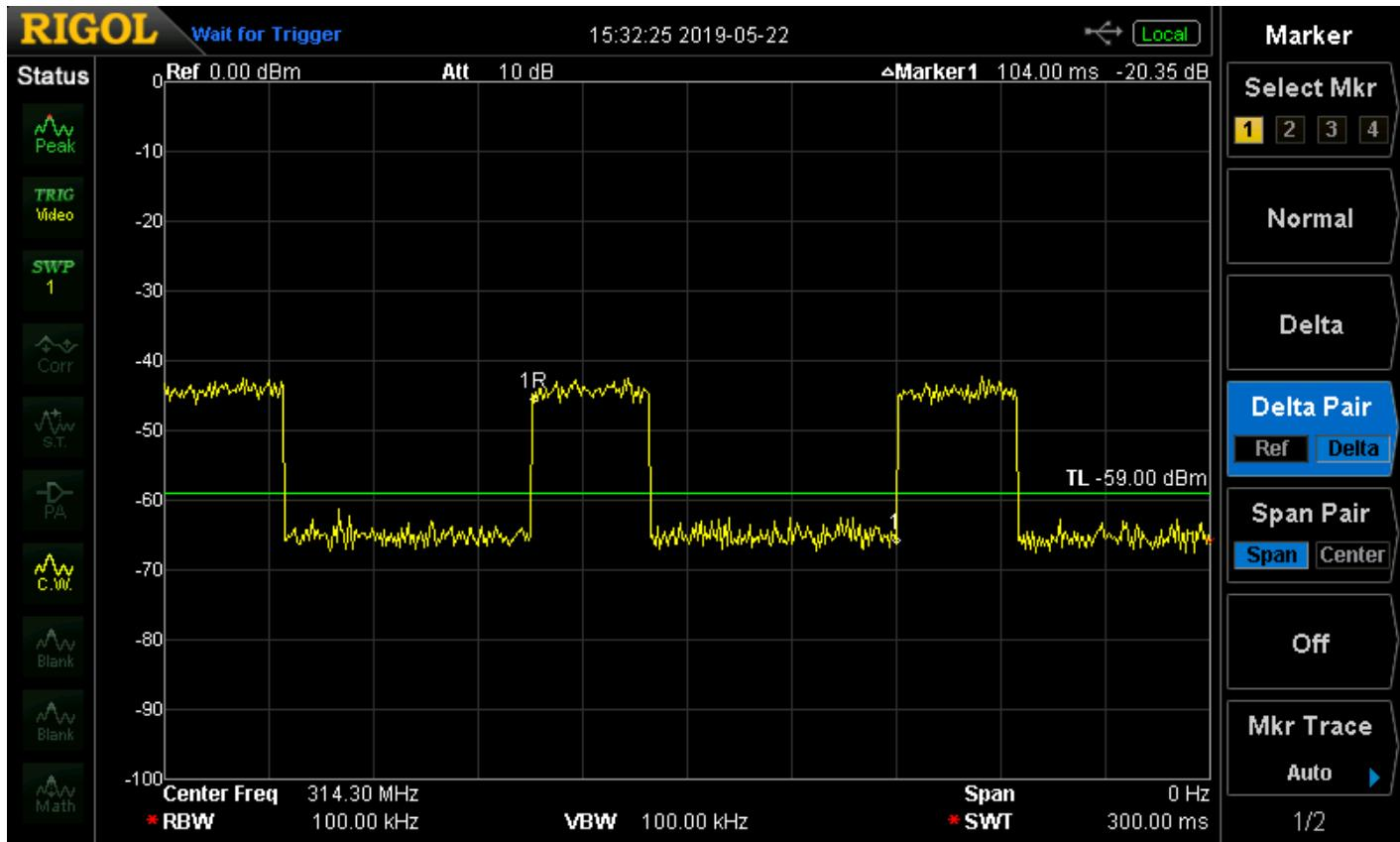
**Test Method: FCC Part 15.231(b)(2), Duty Cycle Determination**
