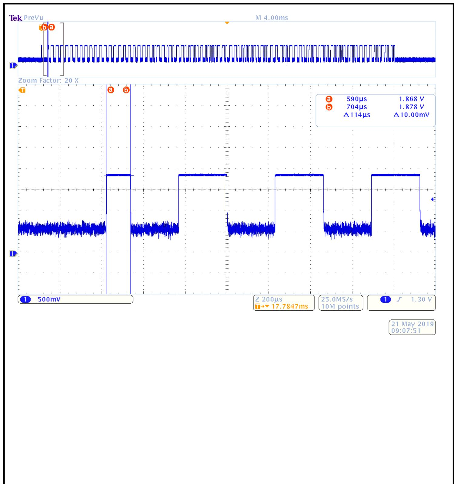
**Test Method: FCC Part 15.231(b)(2), Duty Cycle Determination IC RSS-210 A1.1.2(2) Pulsed Operation**
