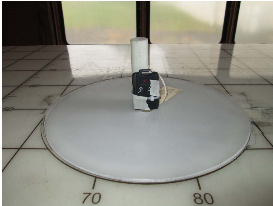
Test Setup, X Axis, Below 1 GHz
