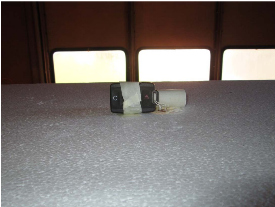
Test Setup, Y Axis, Above 1 GHz
