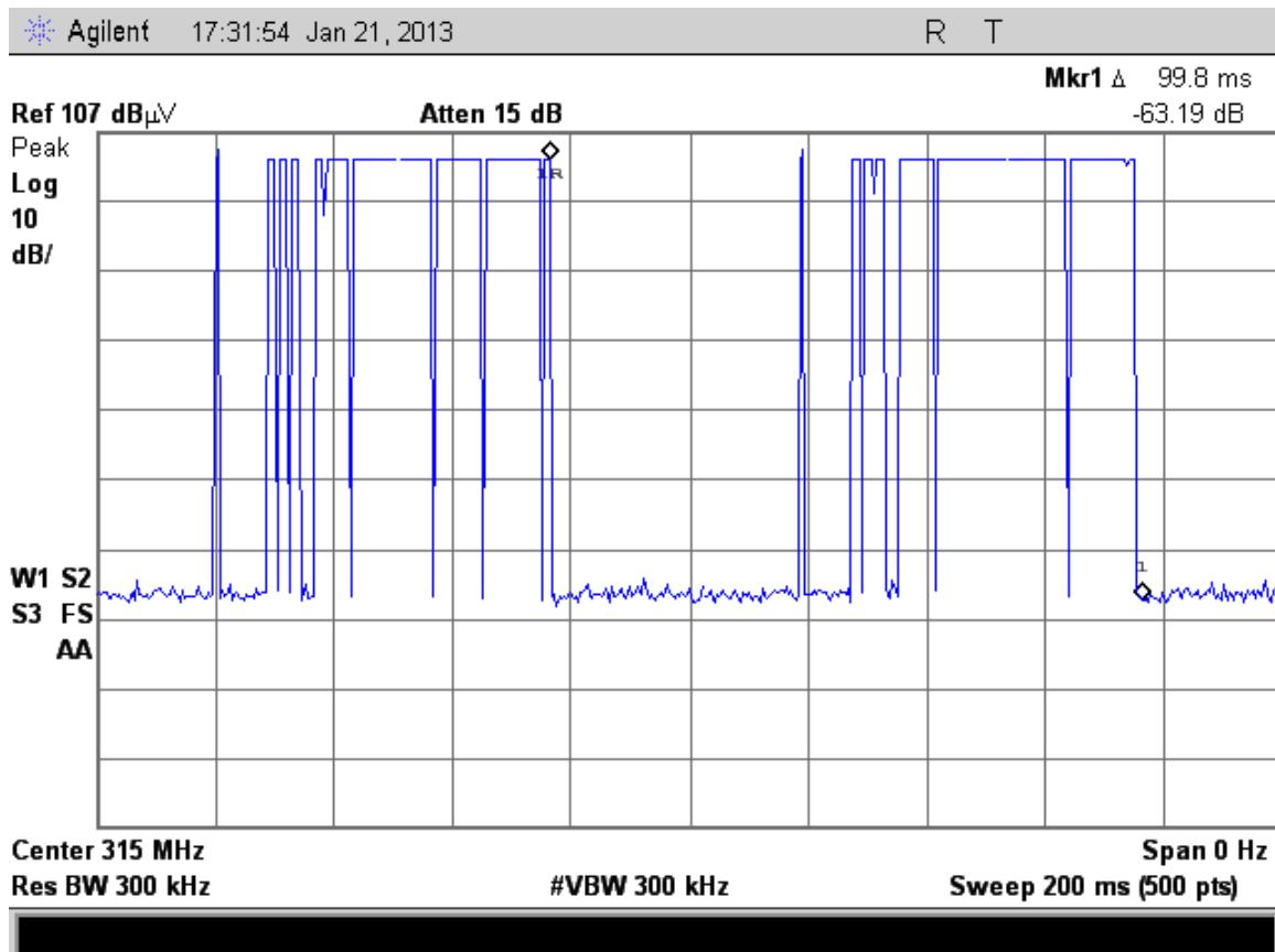
**Test Method: FCC Part 15.231(b), Duty Cycle Determination IC RSS-210 A1.1.2(2) Pulsed Operation**
