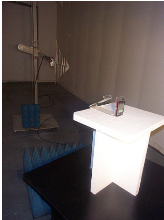
ERP Testing – Vertical Position Configuration #1
