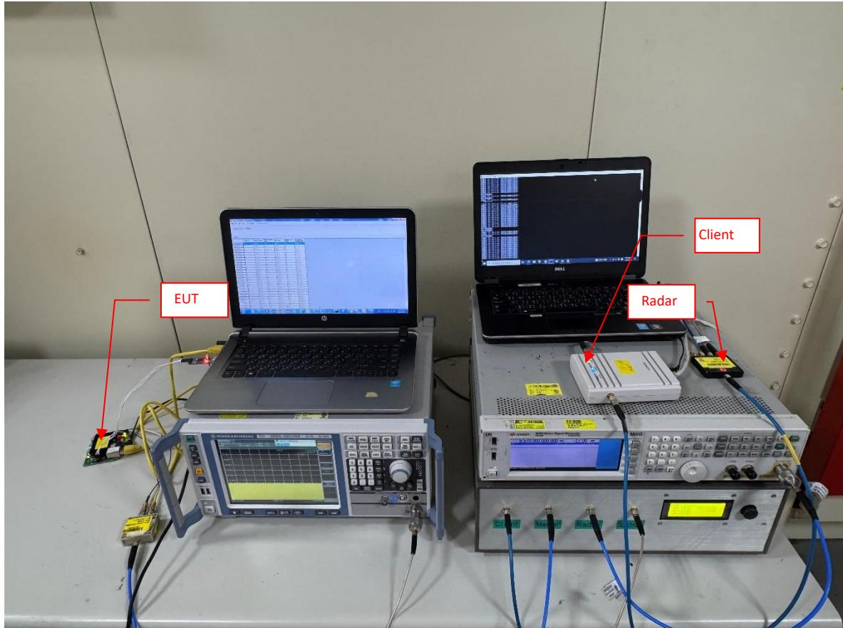
**Set EUT as Client mode (Radar injected into Master)**
