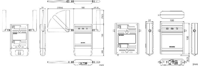
External dimensions (Antenna Connected)
