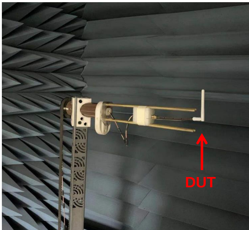
FIGURE 4.1.3 ANTENNA MOUNTED ON 100MM*100MM GROUND PCB TESTED IN OTA CHAMBER
