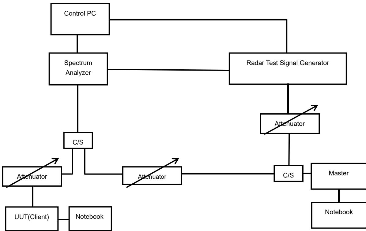
The UUT is a RLAN device operating in Client mode, without Radar Interference Detection function. The radar test signals are injected into the master device.
