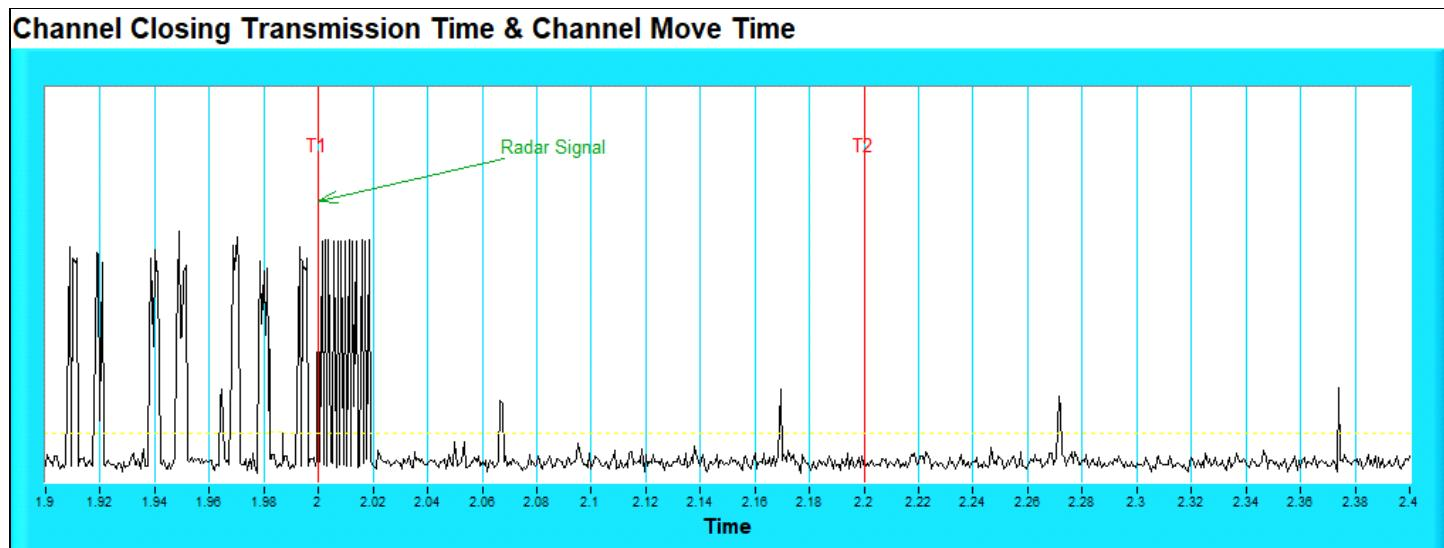
Note: Zoom in of the first 500 ms after radar signal applied.
