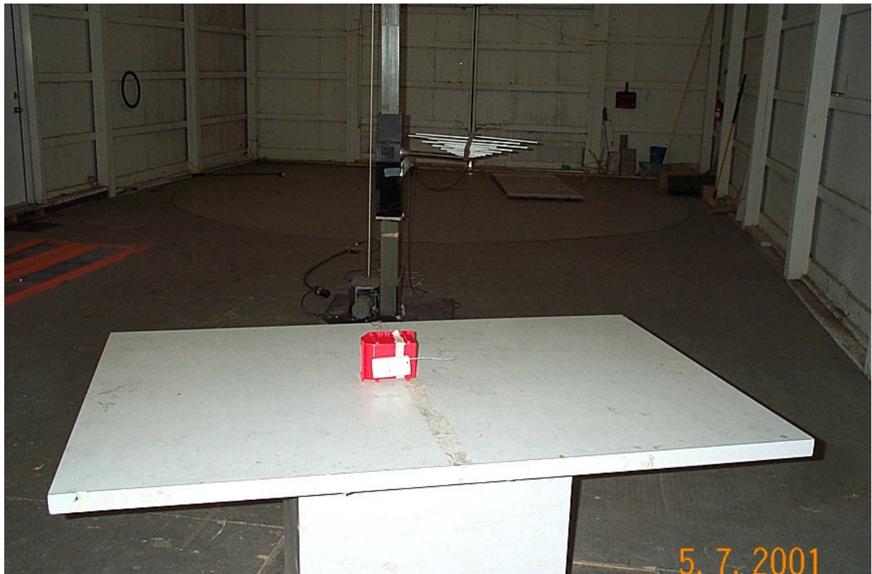
Figure 2. Photograph of Radiated Emissions Test Setup
