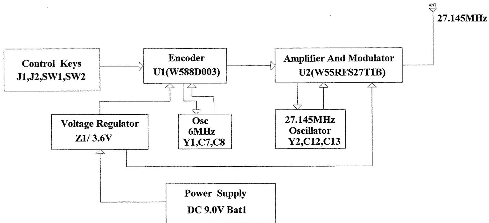
27.145MHz Transmitter Block Diagram
