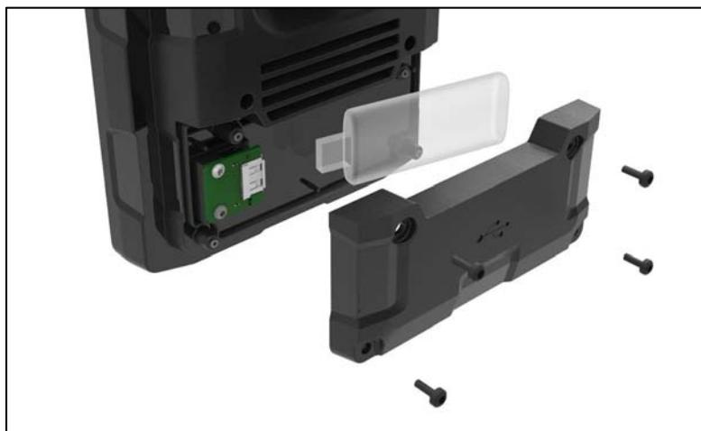
Step #2 - Remove protective cap from the end of the USB Wireless Adapter and insert into the mating connector as shown
