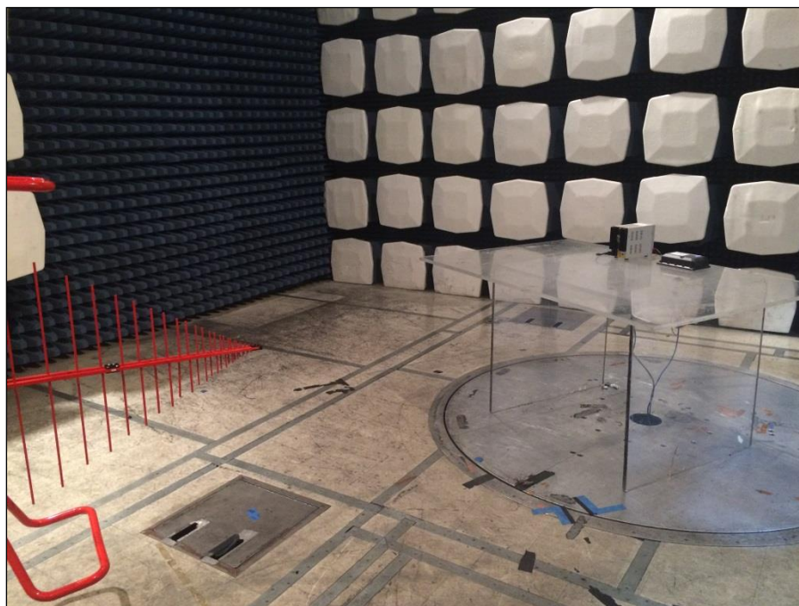
Photograph 1. Undesirable Emissions, Radiated Emission Set up Below 1 GHz
