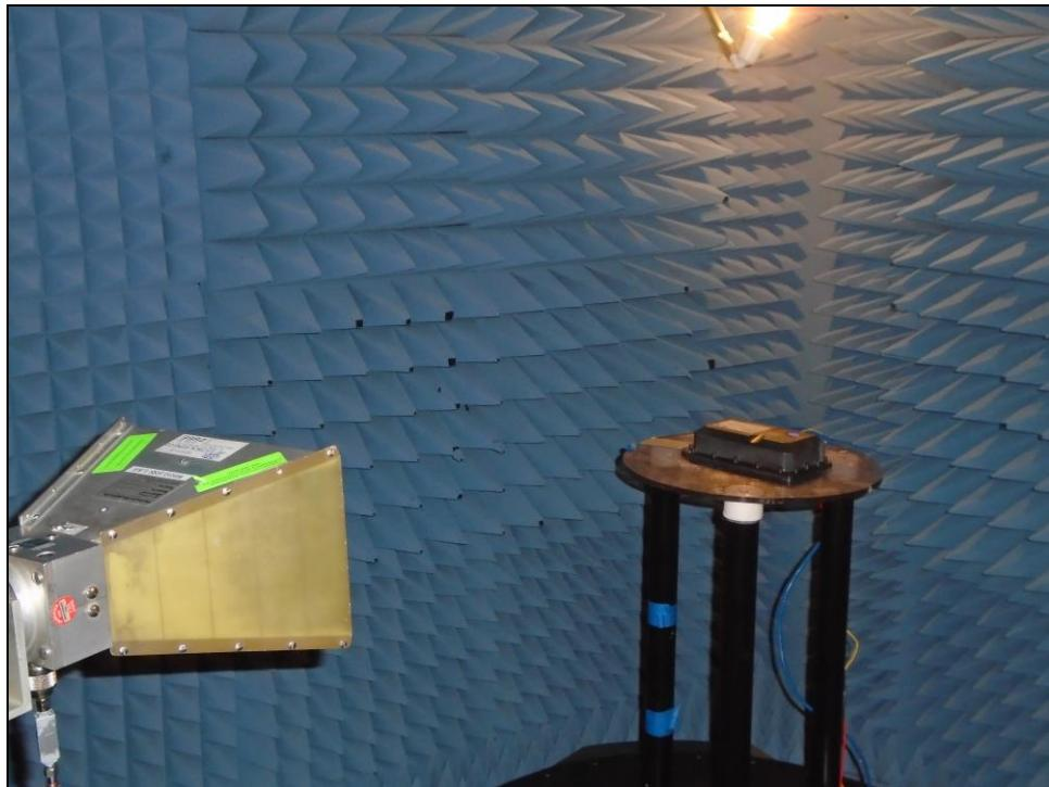
Photograph 1. Undesirable Emissions, Set up Above 1 GHz
