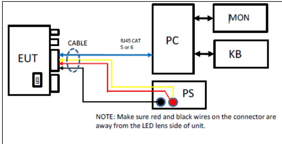
**Figure 1. Block Diagram of Test Configuration 1.1**
