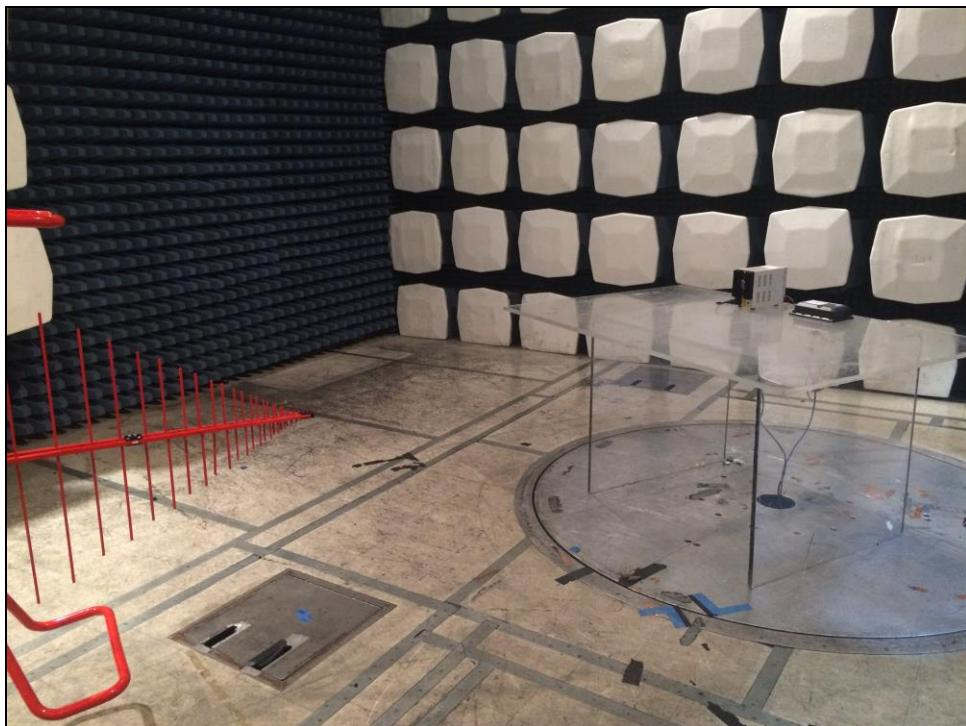
Photograph 2. Undesirable Emissions, Set up Below 1 GHz
