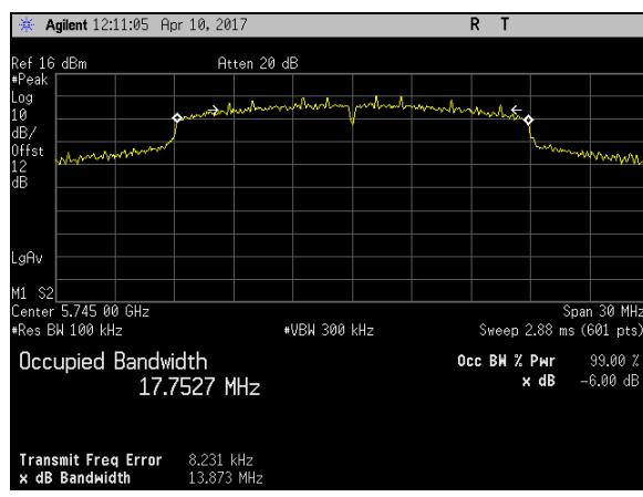
**Plot 107. 6 dB Occupied Bandwidth, BW 20M, Ch 5745M, N Mode Port 1**
