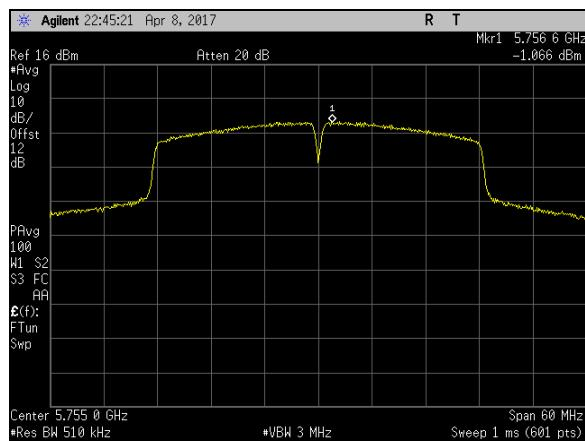
**Plot 30. Power Spectral Density, BW 40M, Ch 5755M, N Mode Port 2**
