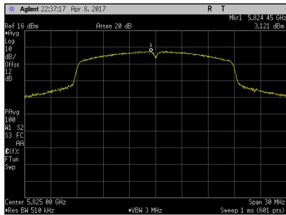
**Plot 28. Power Spectral Density, BW 20M, Ch 5825M, N Mode Port 2**
