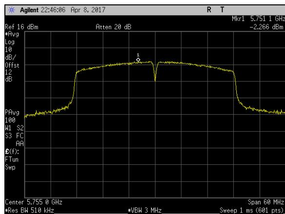
**Plot 29. Power Spectral Density, BW 40M, Ch 5755M, N Mode Port 1**
