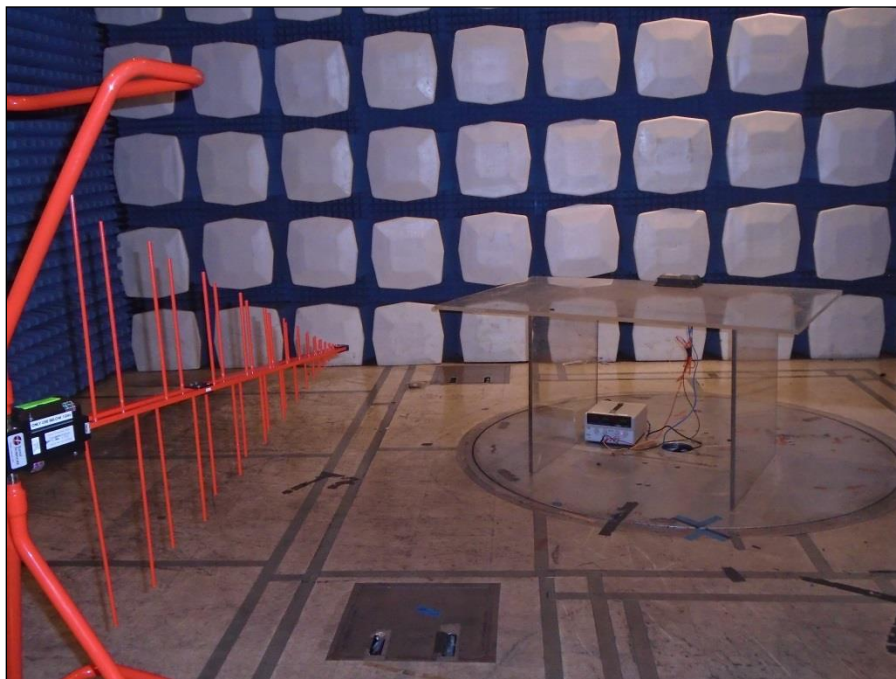
Photograph 2. Spurious Radiated Emissions, up to 1 GHz Test Setup
