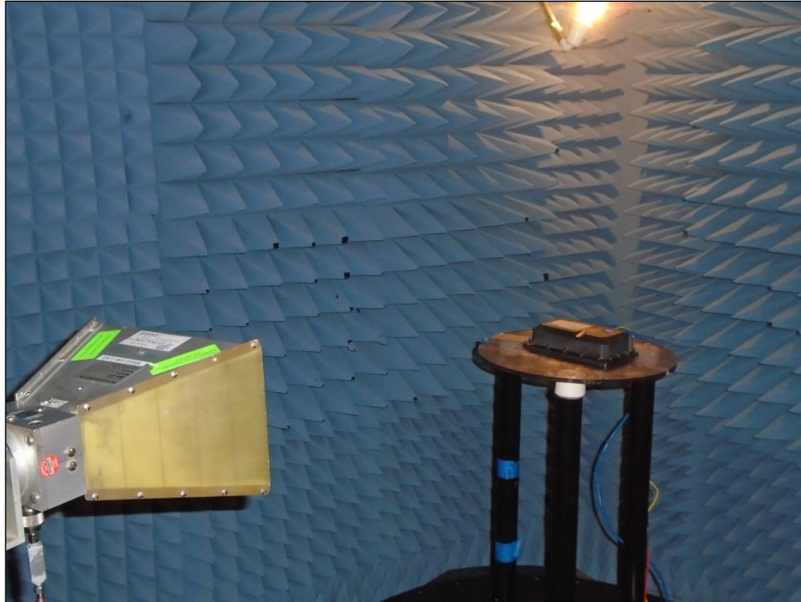
Photograph 1. Spurious Radiated Emissions, above 1 GHz Test setup
