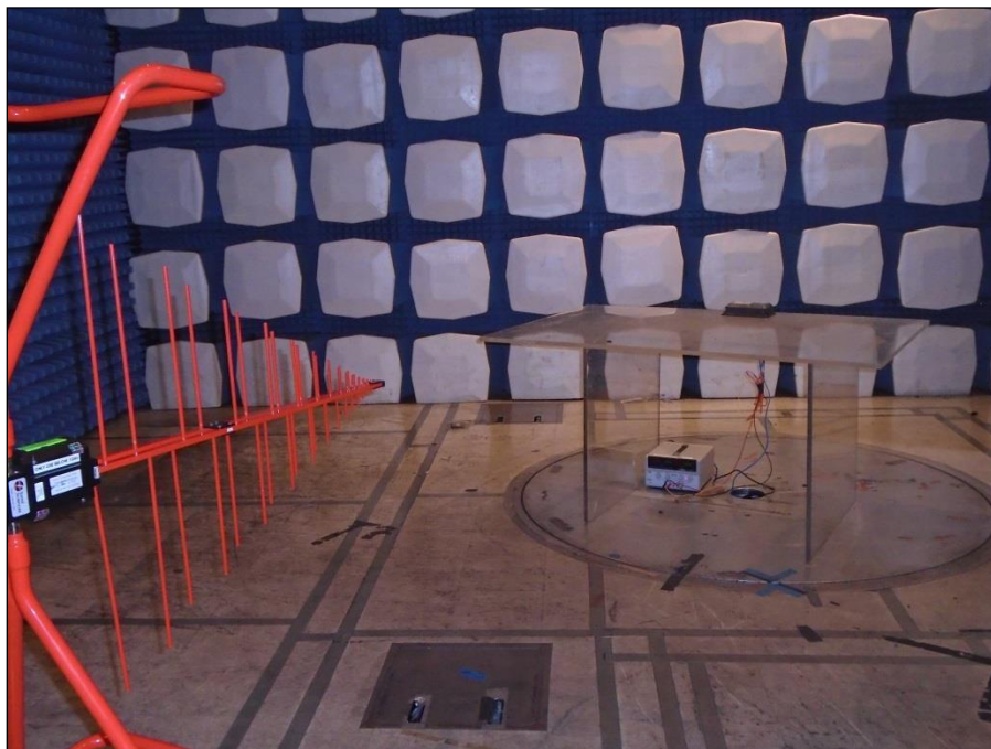
Photograph 2. Spurious Radiated Emissions, up to 1 GHz Test Setup (WiFi)
