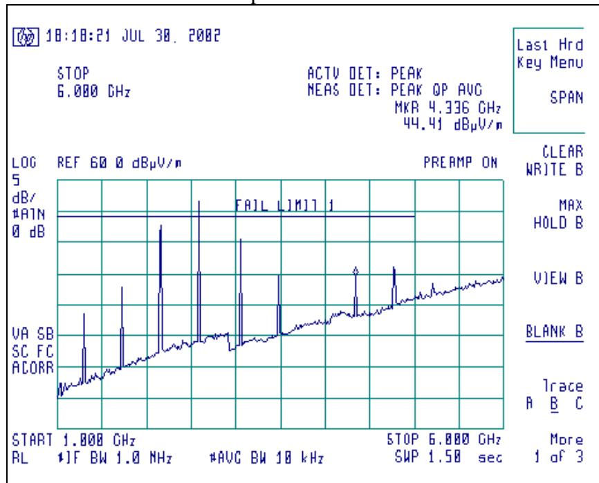
433.92 MHz Signature Scans of the Occupied Bandwidth, with antenna in Horizontal polarization.
