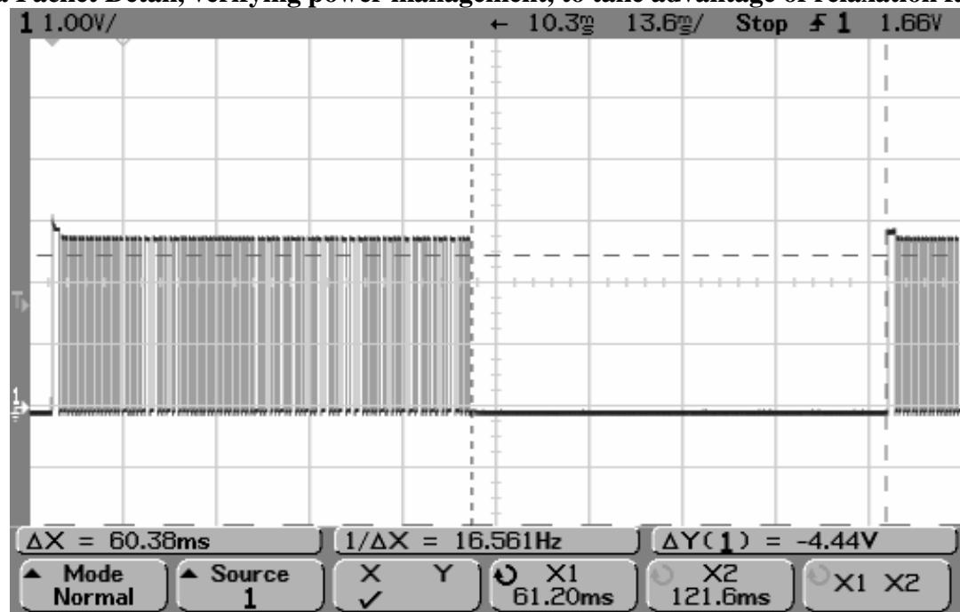
Data Packet Detail, showing transmitted packet, guard time, and power management.
